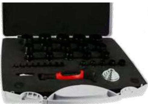
EMPORTE PIÈCE JUMELABLE ET INTERCHANGEABLE. MISE EN PLACE RAPIDE SUR MANDRIN. POUR DÉCOUPER DES RONDELLES OU DES JOINTS DANS LE CAOUTCHOUC, CUIR, CARTON, MOUSSE, PLASTIQUE, TISSU, FIBRE, ALU, CUIVRE. LIVRÉ EN COFFRET DE 10, 15 OU 29 DIAMÈTRES. POINTE DE CENTRAGE RÉTRACTABLE. POIGNÉE BI-MATIÈRE AVEC MANCHE EN ACIER CARBONE BRUNI.
