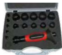
EMPORTE PIÈCE JUMELABLE ET INTERCHANGEABLE. MISE EN PLACE RAPIDE SUR MANDRIN. POUR DÉCOUPER DES RONDELLES OU DES JOINTS DANS LE CAOUTCHOUC, CUIR, CARTON, MOUSSE, PLASTIQUE, TISSU, FIBRE, ALU, CUIVRE. LIVRÉ EN COFFRET DE 10, 15 OU 29 DIAMÈTRES. POIGNÉE BI-MATIÈRE MANCHE ACIER CARBONE BRUNI
