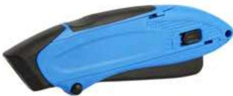
1 FACE ABS - 1 FACE ÉLASTOMÈRE ADHÉRENTE CÔTÉ PAUME. TRÈS BONNE TENUE EN MAIN. SORTIE DE LA LAME PAR PRESSION DES DOIGTS SUR LE LEVIER. RENTRÉE AUTOMATIQUE DE LA LAME DÈS QU'ELLE N'EST PLUS EN ACTION COUPE. BOUTON BLOQUANT LA SORTIE DE LA LAME. LAME MAXI TRAPÈZE. OUVERTURE POUR CHANGEMENT DE LAME PAR GLISSEMENT DU BOÎTIER. SORTIE DE LAME LIMITÉE À 16 MM
