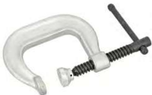
ACIER ÉTIRÉ FORGÉ À HAUTE TENEUR EN CARBONE. CORPS DOUBLE NERVURE. REVÊTEMENT ZINGUÉ. ROTULE, VIS, POIGNÉE REVÊTEMENT NICKEL-CHROME. ROTULE ET PATIN NERVURÉS. VIS À PAS TRAPÉZOÏDAL.
